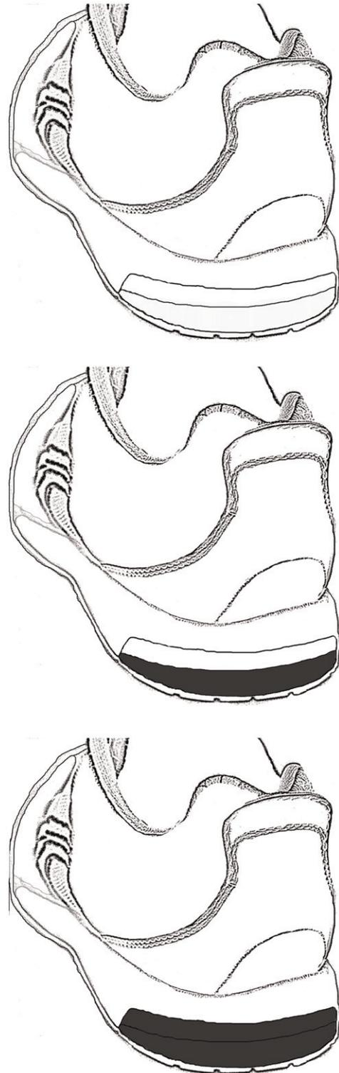
Figure 1. Shoe conditions – crash-pad intervention (LO: 0 mm crash-pad, MI: 10 mm crash-pad, HI: 17 mm crash-pad).
